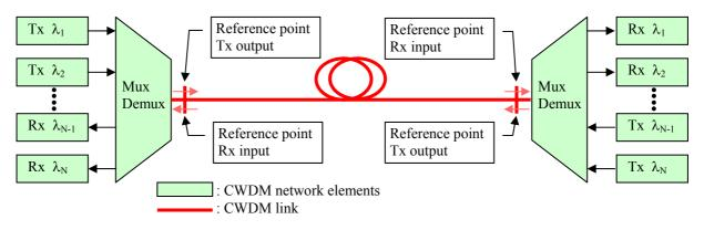
Figure 1. "Black-box" approach for bidirectional applications.
