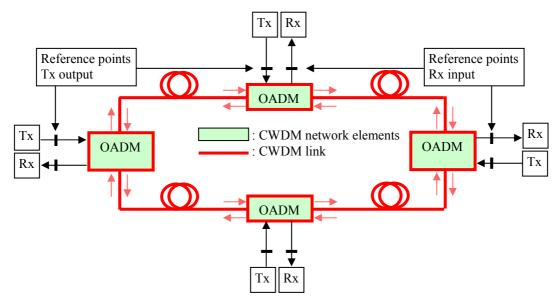
Figure 3. Ring"Black-link" approach for bidirectional applications.
