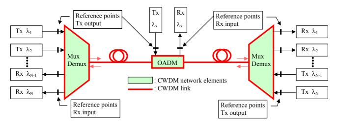
Figure 2. Linear"Black-link" approach for bidirectional applications.
