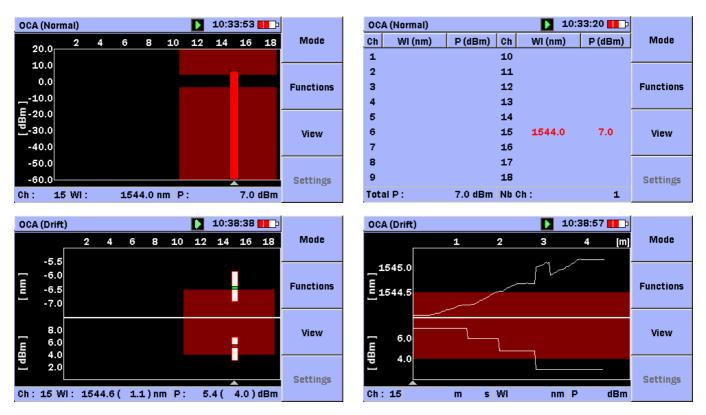
Figure 5. Alarms indicators in the different OCA displays: [top, left]: normal graph display [top, right]: normal table display [bottom, left]: drift graph display [bottom, right]: 1-channel drift plot display
